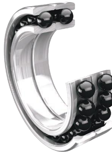
Typical full complement hybrid ceramic pair of bearings for emergency touchdown application.
